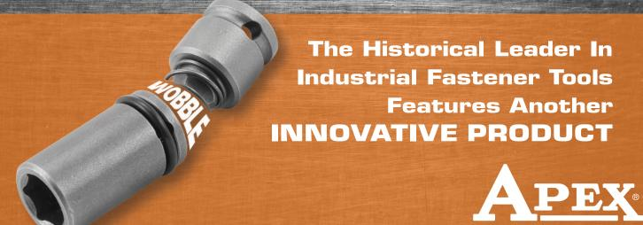
The **Apex WSK Wobble Socket Adapter Kit** can convert any fastener tool with a female square drive (3/8", 1/2", 5/8", 3/4", or 1") and a DIN groove into a Wobble socket. This will enable you to drive fasteners that may have a slight misalignment (up to 10 degrees) between the drive tool axis and the fastener axis. In addition, this will also prove extremely useful in hand-drive operations where clearance may be an issue.
